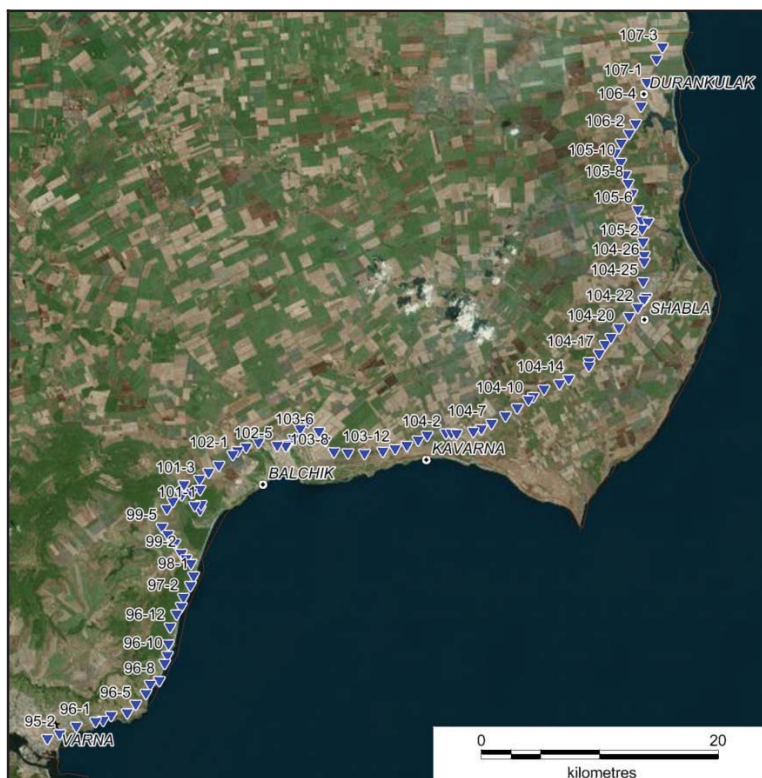
Figure 2. Overview map of the North Black Sea coastline of Bulgaria and location of Route 2 along which are measured the values of the gravity field with a step of 0.250 km between the points.
